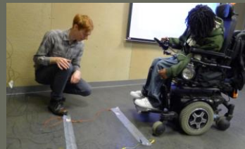
Kevin and Brandon with their prototype showing wheelchair actuated switches that would turn on and off Brandon's lamp in his room.
